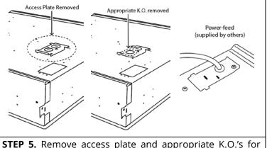
STEP 5. Remove access plate and appropriate K.O.'s for attachment of electrical power feed cable connectors (by others).
