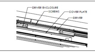
**STEP 4.** Remove and service driver as required. Be sure to wire correctly (both power and dimming, and the wires to LED board). Reinstall cover plate, driver enclosure to reflector assembly, ensure all wires are inside of the driver enclosure. Reinstall reflector and driver enclosure assembly to fixture. Reinstall lens.
