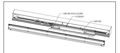
**STEP 3.** Unscrew driver enclosure screws and separate driver enclosure, cover plate from the reflector.
