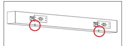
**STEP 2.** Remove the locking screws from wall brackets. Detach the wall mount plates (B) from the luminaire enclosure. Use mounting plate and mounting location diagram to mark location of mounting fasteners (by others).
