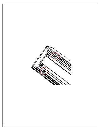
STEP 7. For continuous runs, install Start fixture first (as per steps 1-6). Do not apply power. Remove lens, unscrew the reflector assembly. Lower the reflector / driver enclosure assembly, temporary hung on power cord.
