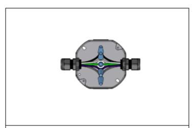
**STEP 6.** Wire fixture using waterproof wire nuts inside junction box (connector/nuts/junction box supplied by others). Refer to provided wiring diagram.
