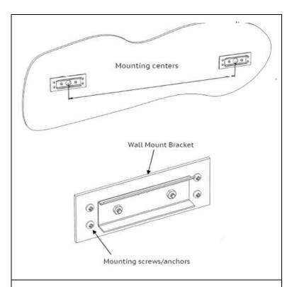
STEP 3. Install wall mounting plates using (4) fasteners for each plate, making sure the plates are installed at the same horizontal level.
