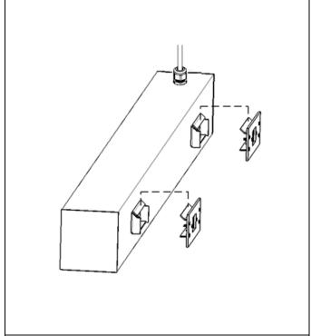
**STEP 4.** Attach luminaire to wall plates.
