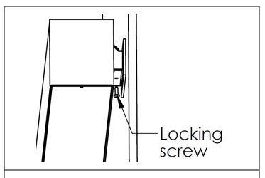
**STEP 5.** Lock fixture to wall mounts by re-attaching locking screws.
