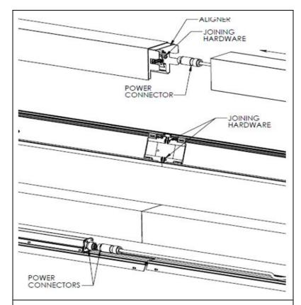
STEP 8. Install joining fixture (as per steps 1-3). Align joining fixture and slide it into place. Then follow steps 4 and 5. Secure with joining hardware. And then connect power connectors together. Reinstall reflector / driver enclosure assembly and lens.
