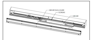
**STEP 3.** Unscrew driver enclosure screws and separate driver enclosure, cover plate from the reflector.
