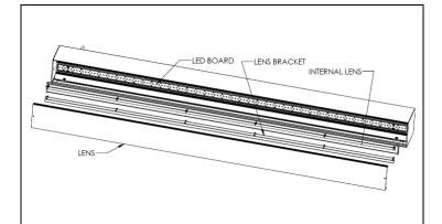
**STEP 1.** For LED board maintenance, remove lens from the unit. Remove the screws and internal lens holding brackets and then remove the internal lens. Remove the screws for LED board and disconnect wires for LED board. Replace LED board and reinstall the screws and wires back. Reinstall internal lens and lens holding brackets and screws. Snap in the external lens back.
