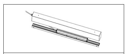
**STEP 4.** Lower the reflector / driver enclosure assembly, temporary hung on power cord.
