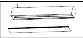
**STEP 2.** Remove the lens from the fixture.
