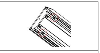
**STEP 3.** Unscrew the reflector assembly.
