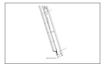
**STEP 5.** Attach fixture to wall (drain holes on bottom) using screws (supplied by others) through the holes in the extrusion. Ensure fixture is secured to a sufficiently strong structure. Reinstall reflector / driver enclosure assembly and lens.
