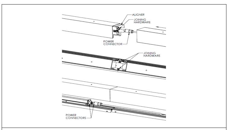
STEP 7. For continuous runs, install Start fixture first (as per steps 1-6). Do not apply power. Install joining fixture (as per steps 1-5). Align joining fixture and slide it into place. Secure with joining hardware. And then connect power connectors together. Reinstall reflector / driver enclosure assembly and lens.
