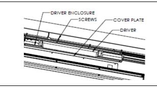
**STEP 4.** Remove and service driver as required. Be sure to wire correctly (both power and dimming, and the wires to LED board). Reinstall cover plate, driver enclosure to reflector assembly, ensure all wires are inside of the driver enclosure. Reinstall reflector and driver enclosure assembly to fixture. Reinstall lens.
