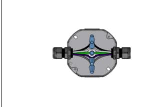
**STEP 6.** Wire fixture using waterproof wire nuts inside junction box (connector/nuts/junction box supplied by others). Refer to provided wiring diagram.
