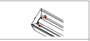
**STEP 3.** Unscrew the reflector assembly.
