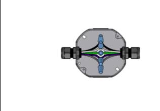
**STEP 6.** Wire fixture using waterproof wire nuts inside junction box (connector/nuts/junction box supplied by others). Refer to provided wiring diagram.
