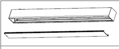
**STEP 2.** Remove the lens from the fixture.
