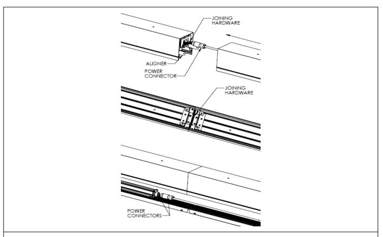
STEP 7. For continuous runs, install Start fixture first (as per steps 1-6). Do not apply power. Install joining fixture (as per steps 1-5). Align joining fixture and slide it into place. Secure with joining hardware. And then connect power connectors together. Reinstall reflector / driver enclosure assembly and lens.
