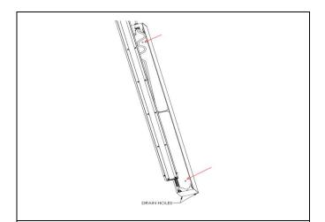
STEP 5. Attach fixture to wall (drain holes on bottom) using screws (supplied by others) through the holes in the extrusion. Ensure fixture is secured to a sufficiently strong structure. Reinstall reflector / driver enclosure assembly and lens.
