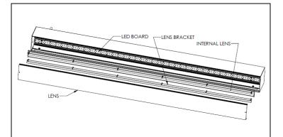
**STEP 1.** For LED board maintenance, remove lens from the unit. Remove the screws and internal lens holding brackets and then remove the internal lens. Remove the screws for LED board and disconnect wires for LED board. Replace LED board and reinstall the screws and wires back. Reinstall internal lens and lens holding brackets and screws. Snap in the external lens back.
