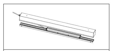
**STEP 4.** Lower the reflector / driver enclosure assembly, temporary hung on power cord.
