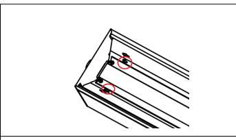
STEP 2. For driver maintenance, remove lens, unscrew the reflector assembly. Lower the reflector / driver enclosure assembly, temporary hung on power cord.
