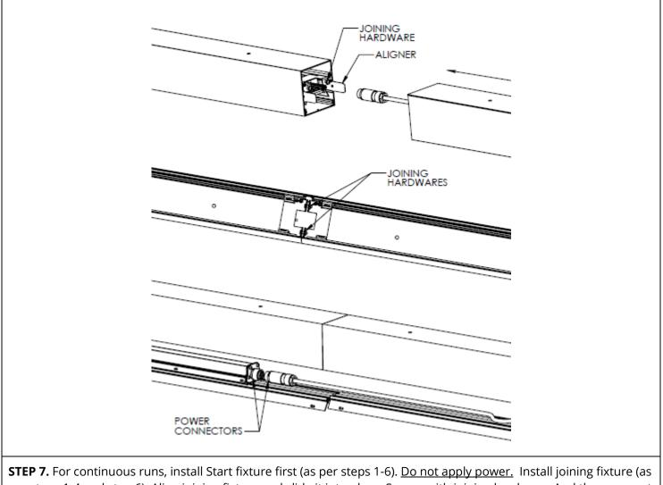
per steps 1-4 and step 6). Align joining fixture and slide it into place. Secure with joining hardware. And then connect power connectors together. Reinstall reflector / driver enclosure assembly and lens.
