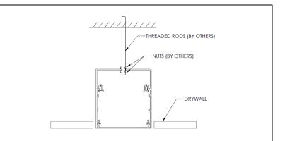
STEP 6. Feed threaded mounting rod (by others) through mounting locations and adjust nut to ensure fixture is parallel to drywall. Insert the fixture all the way through the opening in the ceiling. Insert the second nut (by others) through the fixture and fasten the fixture in place. Repeat with remaining mounting locations until fixture is parallel along entire length. Reinstall reflector / driver enclosure assembly and lens.
