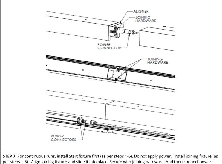
connectors together. Reinstall reflector / driver enclosure assembly and lens.
