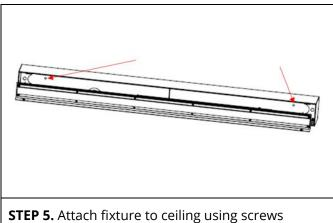
(supplied by others) through the holes in the extrusion. Ensure fixture is secured to a sufficiently strong structure. Reinstall reflector / driver enclosure assembly and lens.
