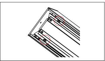
STEP 2. For driver maintenance, remove lens, unscrew the reflector assembly. Lower the reflector / driver enclosure assembly, temporary hung on power cord.
