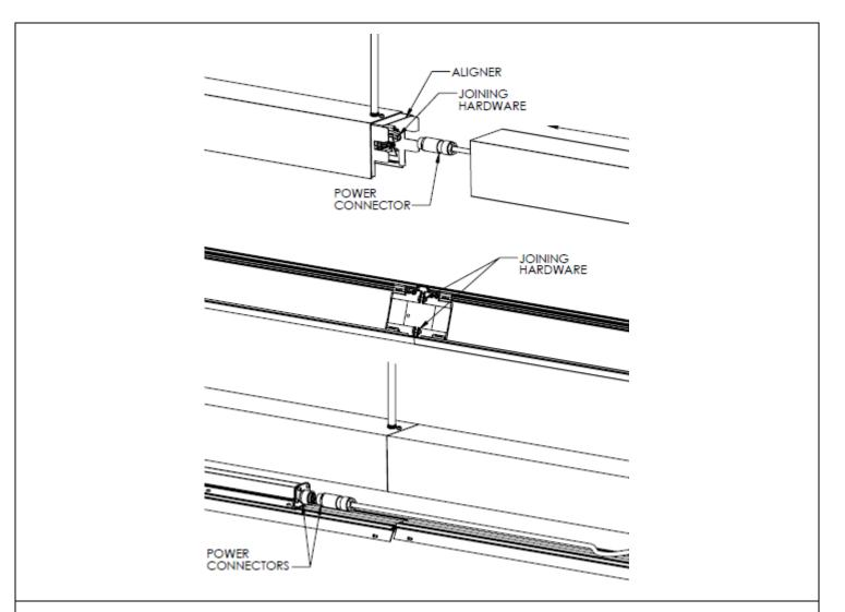
STEP 9. Align joining fixture and slide it into place. Secure with joining hardware. And then connect power connectors together. Reinstall reflector / driver enclosure assembly and lens.
