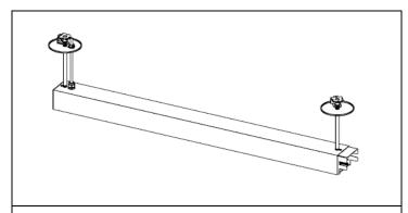
STEP 7. For continuous runs, install Start fixture first (as per steps 1-6). Do not apply power.
