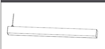
STEP 1. Remove fixture and solid stem kits packaging, note marked supply power cord coming out at the top of the luminaire.
