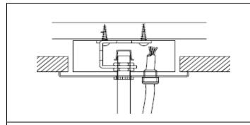
**STEP 6.** Adjust hex nuts and stems as needed to level fixture and then tighten the nuts. Adjust and lock canopy in place by tightening the set screw in the slip ring under canopy.
