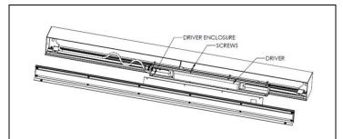
**STEP 3.** Unscrew driver enclosure screws and separate driver enclosure, cover plate from the reflector.
