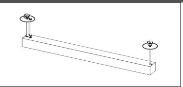
**STEP 2.** Attach stems to threaded holes at the top of the luminaire enclosure - one at each end, install power cord to the connector in the canopy.
