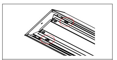
STEP 8. Remove lens from the fixture. Unscrew the reflector assembly. Lower the reflector / driver enclosure assembly, temporary hung on power cord.
