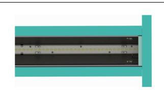
**STEP 8.** Place the reflector assembly back into the fixture and fasten with the same 4 screws taken out. Repeat for each reflector assembly to be reinstalled.
