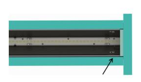
STEP 5. Remove reflector mounting screws (4 per reflector) and reflector/LED assembly. Note that fixtures with an optional emergency pack may have a test switch and indicator light mounted on the reflector.
