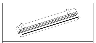
**STEP 2.** Remove the lens from the fixture.
