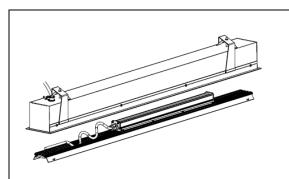
**STEP 5.** Install BX connector (supplied by others). Feed BX cable (supplied by others) through connector and the body enclosure. Tighten BX connector screw. Wire power cord to BX cable using waterproof wire nuts (supplied by others). Refer to provided wiring diagram.
