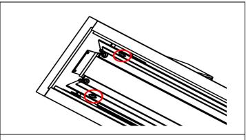
**STEP 3.** Unscrew the reflector assembly.
