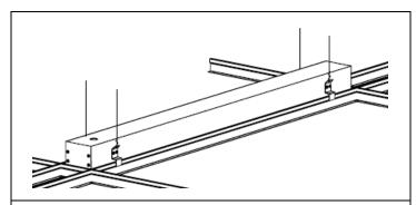
**STEP 2.** Place luminaire into ceiling and rest it onto the T-bar. Center and secure fixture to structure above by attaching security wires (by others) to holes at the hanger brackets.
