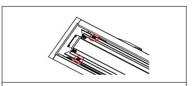
**STEP 4.** Unscrew the reflector assembly.
