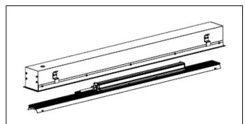
STEP 5. Lower the reflector / driver enclosure assembly
