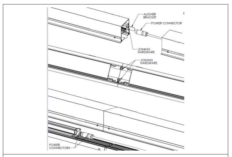
STEP 7. For continuous runs, install Start fixture first (as per steps 1-6). Do not apply power. Install joining fixture (as per steps 1-5). Align joining fixture and slide it into place. Secure with joining hardware. And then connect power connectors together. Reinstall reflector / driver enclosure assembly and lens.
