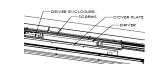
**STEP 4.** Remove and service driver as required. Be sure to wire correctly (both power and dimming, and the wires to LED board). Reinstall cover plate, driver enclosure to reflector assembly, ensure all wires are inside of the driver enclosure. Reinstall reflector and driver enclosure assembly to fixture. Reinstall lens.
