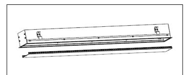
**STEP 3.** Remove the lens from the fixture.
