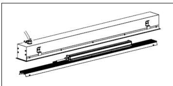
**STEP 6.** Install BX connector (supplied by others). Feed BX cable (supplied by others) through connector and the body enclosure. Tighten BX connector screw. Wire power cord to BX cable using waterproof wire nuts (supplied by others). Refer to provided wiring diagram. Reinstall reflector / driver enclosure assembly and lens.
