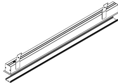
**STEP 2.** Remove the lens from the fixture.
