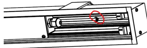
**STEP 6.** Insert fixture into drywall cutout in ceiling. Attach fixture to ceiling by turning the screws attached to the drywall brackets. The brackets will rotate over the drywall to secure the fixture.
