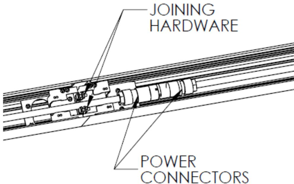
**STEP 7.** For continuous runs, install Start fixture first (as per steps 1-6). Do not apply power. Install joining fixture (as per steps 1-4 and step 6). Align joining fixture and slide it into place, then follow step 6 to secure the fixture to drywall and then install the joining hardware. Then connect power connectors together. Reinstall reflector assembly and lens.
