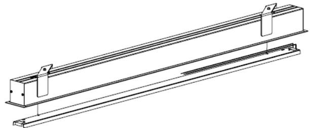
**STEP 4.** Lower the reflector assembly, hung on safety cables or wires.
