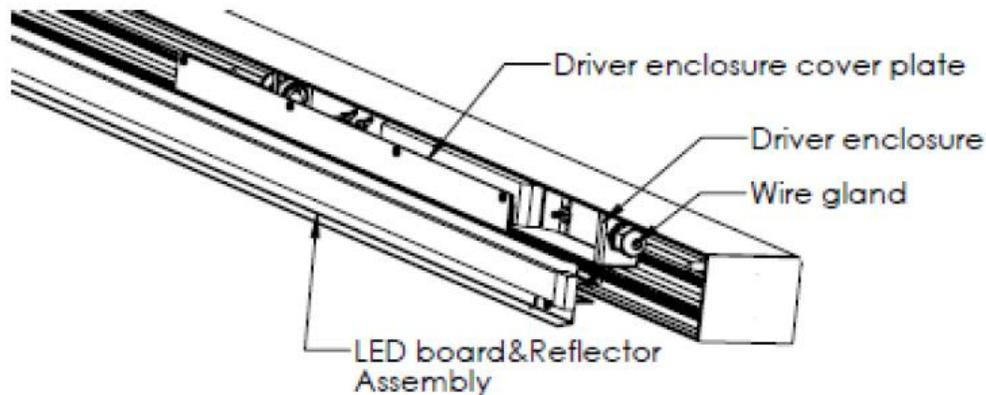
Remove lens from the unit. Remove screws from the reflector assembly. Lower the reflector assembly, hung on safety cable. Remove the screws and then remove the driver enclosure cover plate.
