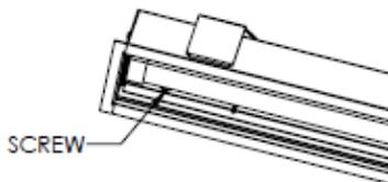
**STEP 3.** Unscrew the reflector assembly.
