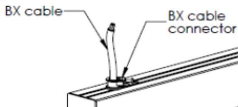
**STEP 5.** Install BX connector (supplied by others). Feed BX cable (supplied by others) through connector and the body enclosure. Tighten BX connector screw. Wire power cord to BX cable using waterproof wire nuts (supplied by others). Refer to provided wiring diagram.
