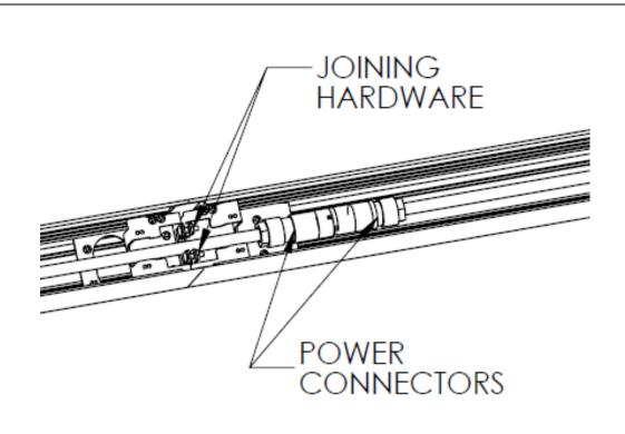
STEP 7. For continuous runs, install Start fixture first (as per steps 1-6). Do not apply power. Install joining fixture (as per steps 1-4). Align joining fixture and slide it into place, then follow step 6 to secure the fixture to threaded rod and then install the joining hardware. Then connect power connectors together. Reinstall reflector assembly and lens.
