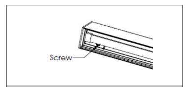
**STEP 3.** Remove screws from the reflector assembly.
