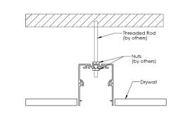
**STEP 6.** Feed threaded mounting rod (by others) through mounting locations and adjust nut to ensure fixture is parallel to drywall. Insert the fixture all the way through the opening in the ceiling. Insert the second nut (by others) through the fixture and fasten the fixture in place. Repeat with remaining mounting locations. Reinstall reflector assembly and lens.
