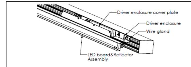
Remove lens from the unit. Remove screws from the reflector assembly. Lower the reflector assembly, hung on safety cable. Remove the screws and then remove the driver enclosure cover plate.
