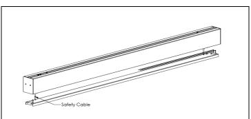
**STEP 4.** Lower the reflector assembly, hung on safety cable.
