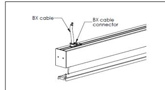
**STEP 5.** Install BX connector (supplied by others). Feed BX cable (supplied by others) through connector and the body enclosure. Tighten BX connector screw. Wire power cord to BX cable using waterproof wire nuts (supplied by others). Refer to provided wiring diagram.
