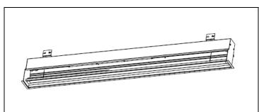
**STEP 2.** Remove lens from the fixture. Unscrew the reflector assembly. Lower the reflector assembly, hung on safety cables or wires.
