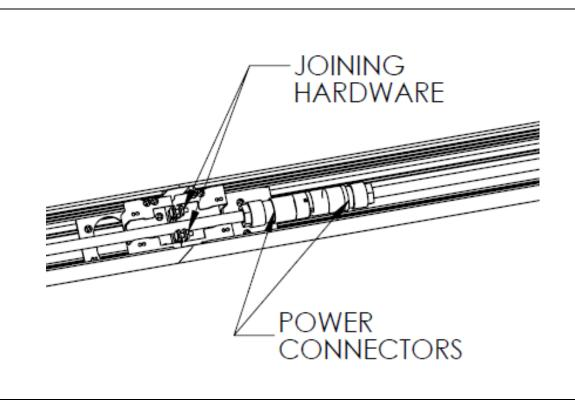
**STEP 6.** For continuous runs, install Start fixture first (as per steps 1-4). <u>Do not apply power.</u> Prepare joining fixture (as per steps 1 and 2). Align joining fixture and slide it into place, then follow step 4 to secure the fixture and then install the joining hardware. Then connect power connectors together. Reinstall reflector assembly and lens. Then follow step 5 to finish the ceiling.
