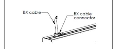
STEP 3. Install BX connector (supplied by others). Feed BX cable (supplied by others) through connector and the body enclosure. Tighten BX connector screw. Wire power cord to BX cable using waterproof wire nuts (supplied by others). Refer to provided wiring diagram.
