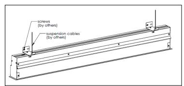
**STEP 4.** Install luminaire to wall, be sure top of the flange is the same level of ceiling. Secure suspension cables to holes on the wall bracket.
