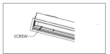
**STEP 3.** Remove screws from the reflector assembly.
