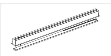
**STEP 4.** Lower the reflector assembly, hung on safety cable.
