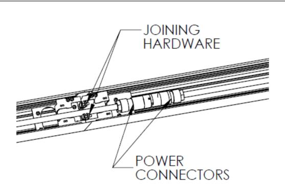
STEP 7. For continuous runs, install Start fixture first (as per steps 1-6). Do not apply power. Install joining fixture (as per steps 1-4). Align joining fixture and slide it into place, then follow step 6 to secure the fixture to threaded rod and then install the joining hardware. Then connect power connectors together. Reinstall reflector assembly and lens.
