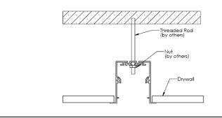
**STEP 6.** Feed threaded mounting rod (by others) through mounting locations. Insert the fixture all the way through the opening in the ceiling. Insert nut (by others) through the fixture and fasten the fixture in place. Repeat with remaining mounting locations. Reinstall reflector assembly and lens.
