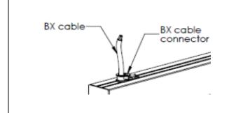
**STEP 5.** Install BX connector (supplied by others). Feed BX cable (supplied by others) through connector and the body enclosure. Tighten BX connector screw. Wire power cord to BX cable using waterproof wire nuts (supplied by others). Refer to provided wiring diagram.
