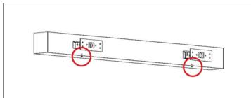
**STEP 2.** Remove the locking screws from wall brackets. Detach the wall mount plates from the luminaire enclosure. Use mounting plate and mounting location diagram to mark location of mounting fasteners (by others).
