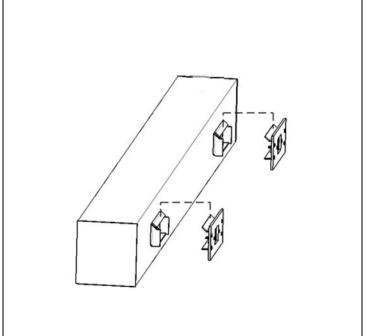
**STEP 4.** Attach luminaire to wall plates.
