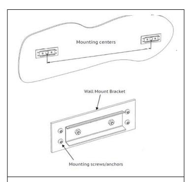
**STEP 3.** Install wall mounting plates using (4) fasteners for each plate, making sure the plates are installed at the same horizontal level.
