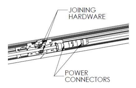
STEP 7. For continuous runs, install Start fixture first (as per steps 1-6). Do not apply power. Install joining fixture (as per steps 1-3, remove lens, unscrew the reflector assembly, lower the reflector assembly, temporary hung on safety cable. Align joining fixture and slide it into place, then follow steps 4-5 to secure the fixture to wall. Install joining hardware. Then connect power connectors together. Reinstall reflector assembly and lens.
