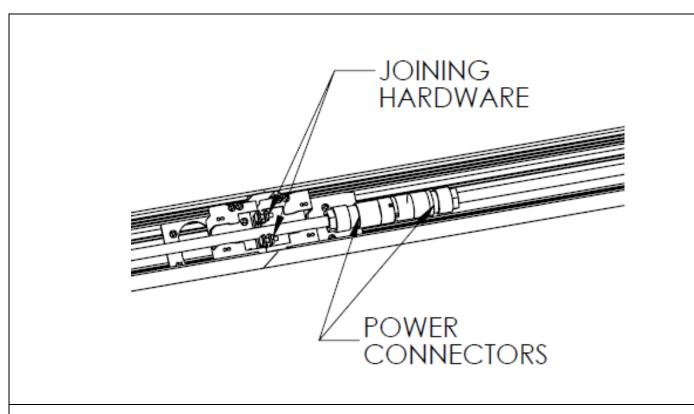
STEP 7. For continuous runs, install Start fixture first (as per steps 1-6). Do not apply power. Install joining fixture (as per steps 1-4). Align joining fixture and slide it into place, then follow step 5 to secure the fixture to wall. Install joining hardware. Then connect power connectors together. Reinstall reflector assembly and lens.
