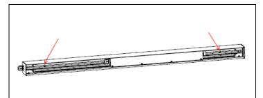
**STEP 5.** Attach fixture to wall vertically using screws (supplied by others) through the holes in the extrusion, ensuring the wire entry is on the top (noted the drain holes are at the bottom). Ensure fixture is secured to a sufficiently strong structure.
